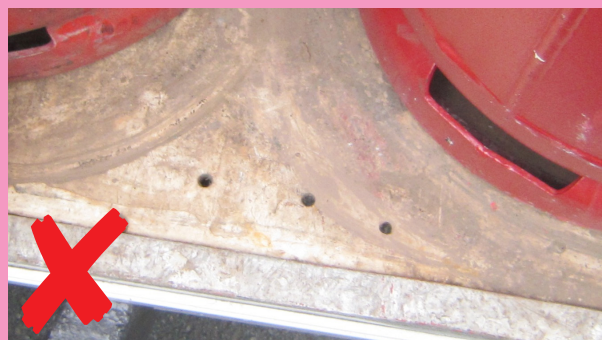
Ventilation holes in the base of the cylinder compartment.
