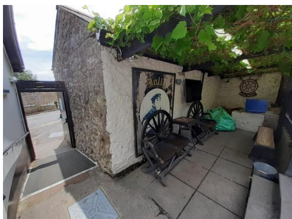
LEFT - INDOOR TELEVISION MOUNTED ON AN EXTERNAL WALL UNDER A CANOPY. RIGHT - INDOOR TELEVISION IN A PARTIALLY ENCLOSED AREA WITH AN INDOOR EXTENSION LEAD ON THE WALL TO THE UPPER RIGHT OF THE TELEVISION.
